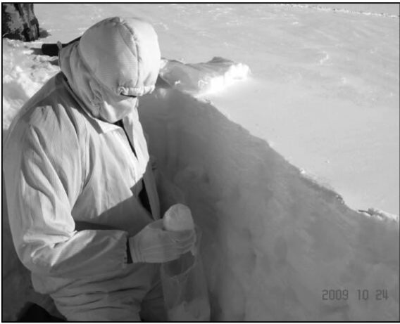
图 3 雪坑采样 Fig. 3 A photo showing snow sampling in a snowpit
