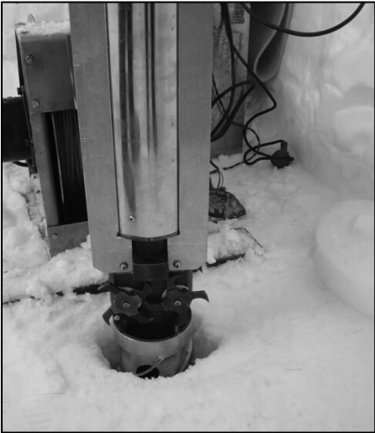
图 4 冰芯的钻取 Fig. 4 A photo showing extractor of ice core
