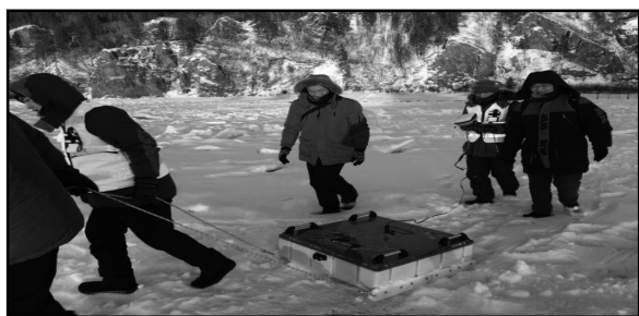
图2 GPR-10型冰厚、水深雷达同步测量系统测试现场 Fig. 2 Photo showing the GPR-10 ice thickness and water depth radar synchronous measuring system
