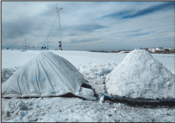
图2 高山区气象观测场附近的储雪实验 Fig. 2 Snow storage near the meteorological observation site in alpine region
