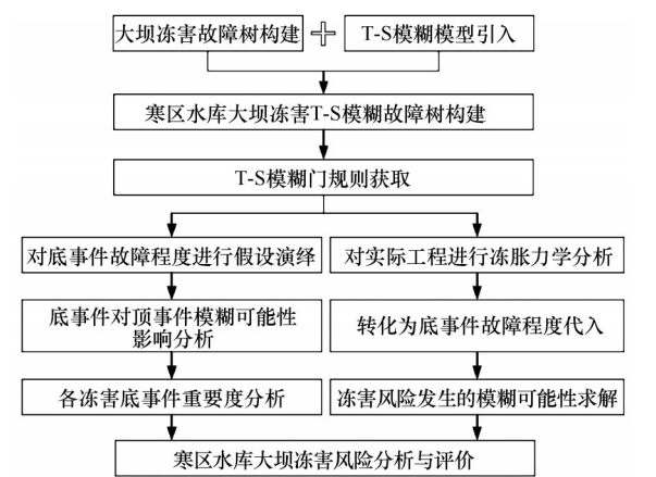
图5 基于T-S模糊故障树的水库大坝冻害风险分析流程 Fig. 5 Frost damage risk analysis process of reservoir dam based on T-S fuzzy fault tree
